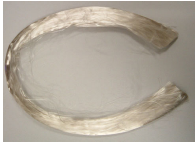
Fig. 1 Fibre tow obtained using a specially made in-house fibre production facility
